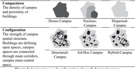
Figure 1: Compactness and configuration of a well-designed campus Source: Hajrasouliha, 2017
