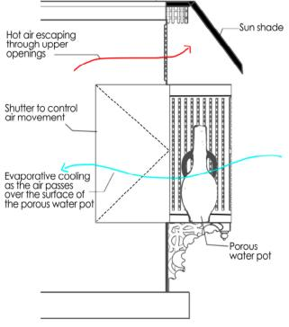
Figure 1: Indoor air-cooling system created by placing porous water jars in the Mashrabiya. Source: (Taki & Kumari, 2023)
