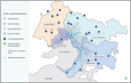
Figure 5: Melbourne sanitation System Source: Melbourne Sewerage Strategy, (2022)
