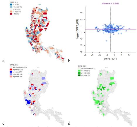
Figure 7: Deviation from the predicted LSR dependency of LGUs in Luzon Island during 2021 (a) Chloropleth Map, (b) Moran's Scatterplot, (c) LISA Cluster Map, and (d) Significance Map Source: Map produced using GeoDa software (version 1.20)
