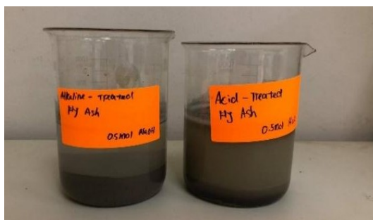
Figure 1: Fly ash soaked in HCl and NaOH
