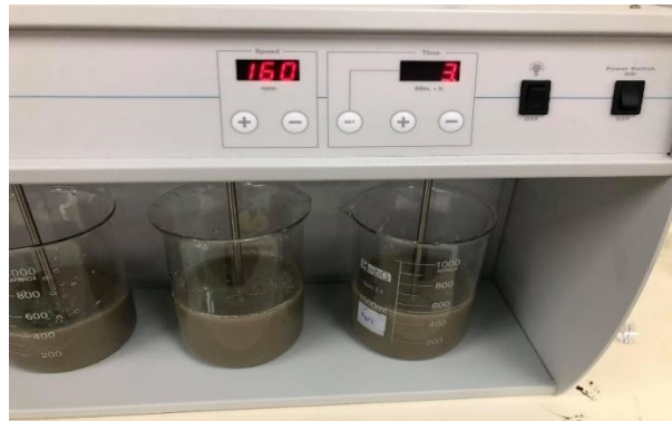
Figure 2: Jar test apparatus and setting
