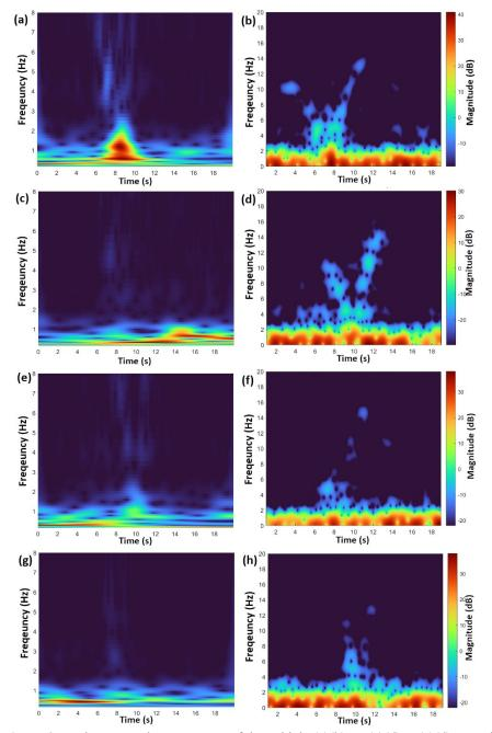
**Figure 3:** Scalogram and spectrogram of the vehicle (a)(b) A, (c)(d) B,(c)(d) C, and (e)(f) D, respectively, with an operating frequency of 434 MHz
