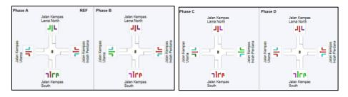
Figure 3: Jalan Kempas intersection phasing plan according to current cycle time
