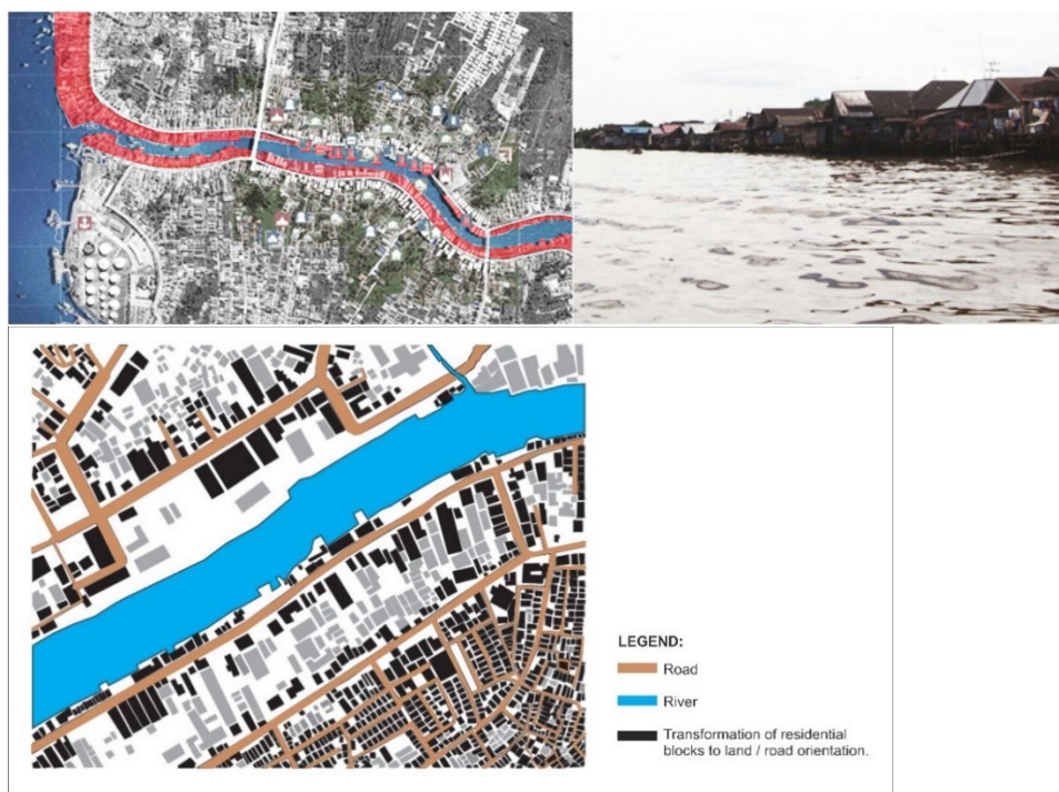
Figure 6. Road-Oriented Settlement Transformation/Land Based due to Urban Planning (bottom) and before (top) (drawn by Yustina)
