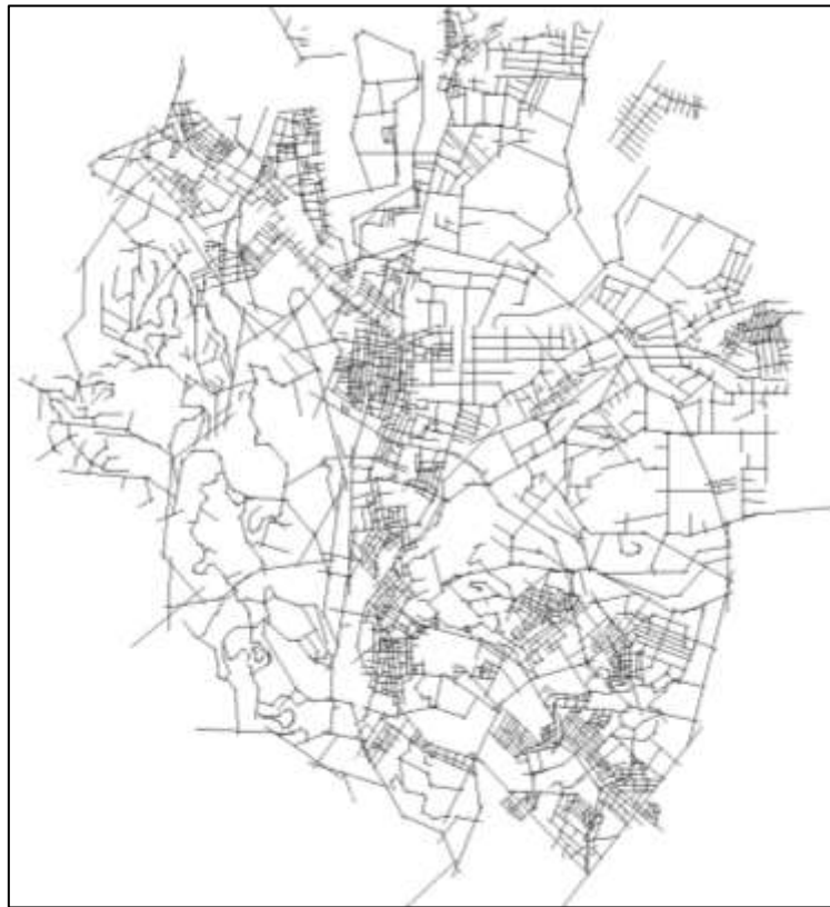
Figure 3: The Axial map consists of 2,437 street segments that were audited in the DepthMap software
