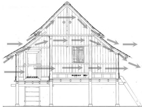
Figure 1: Ventilation Openings in the Roof of Traditional Malay House
