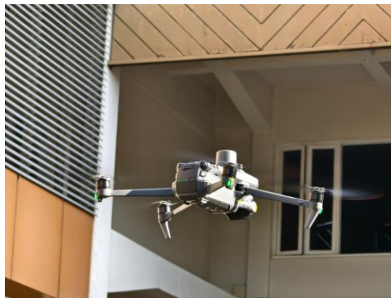
Figure 3: UAV platform used for rooftop thermal image acquisition
