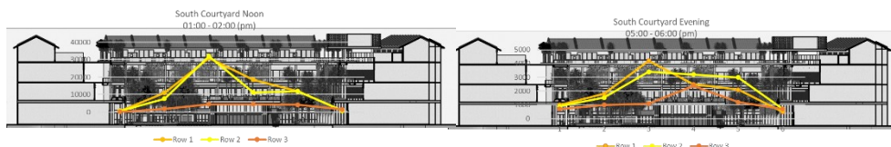
Figure 12: Lux level at South courtyard at noon and evening
