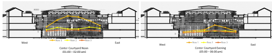
Figure 10: Lux level at Centre courtyard at noon and evening
