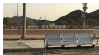
Figure 4.6: Aluminum bench material is unsuitable for hot and humid climate
