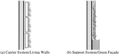
(a) Carrier System/Living Walls (b) Support System/Green Façade **Figure 1**: Vertical Greenery Systems *Source: Tan et al.* (2009)
