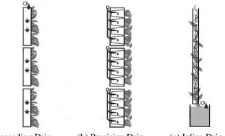
(a) Cascading Drip (b) Precision Drip (c) Inline Drip **Figure 3**: Irrigation systems for vertical greeneries *Source: Tan et al.* (2009)
